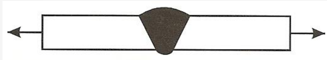
Junta topo a topo transversal
