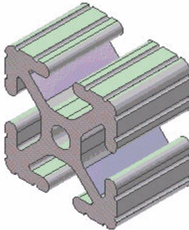
**Figure 1 - Aluminum Extrusion Model**
