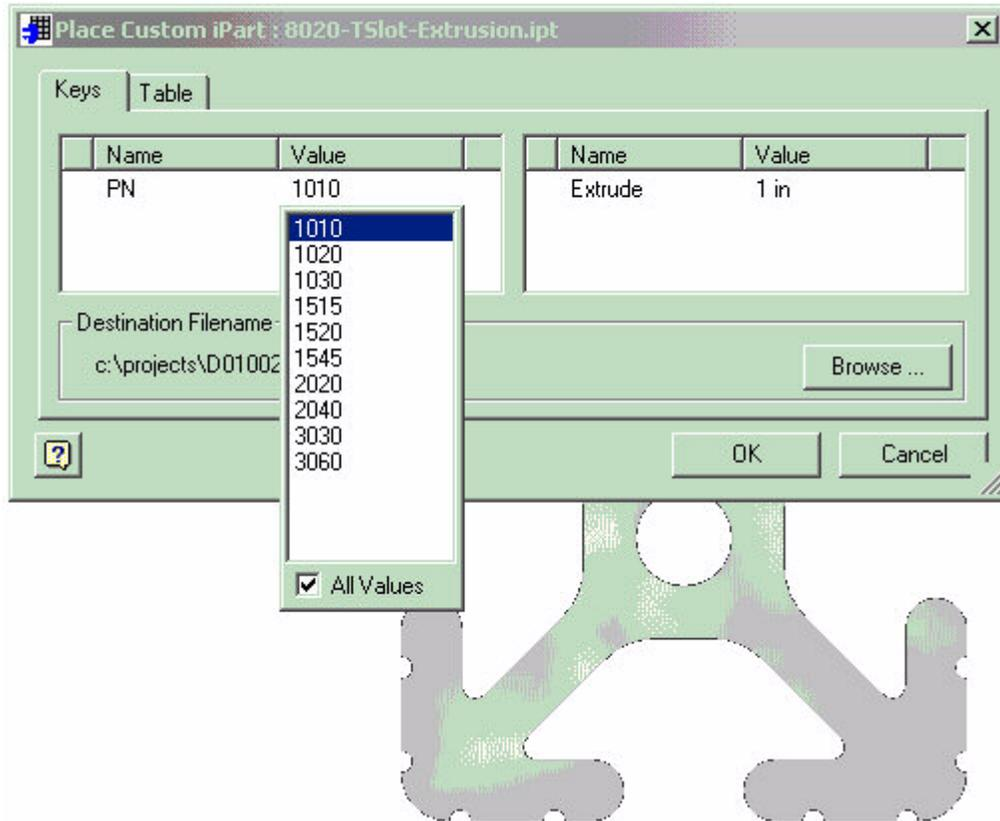
Figure 5 – Inserting iPart, Value Keys Reflected
