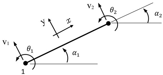
$$\begin{Bmatrix} v_1 \\ \theta_1 \\ v_2 \\ \theta_2 \end{Bmatrix} = [R]_V \begin{Bmatrix} U_1 \\ U_2 \\ U_3 \\ U_4 \\ U_5 \\ U_6 \end{Bmatrix}$$
