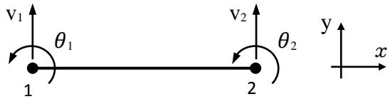
$$V(x) = \frac{dM(x)}{dx} \quad M(x) = EI_z \frac{d^2v(x)}{dx^2} \quad \sigma_x(x, y) = -\frac{M(x) \cdot y}{I_z}$$
