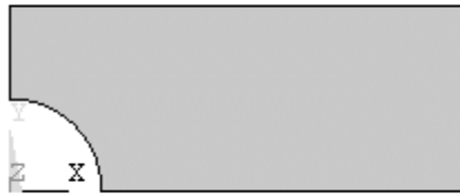
Figure 2-11 Geometry for quadrant of plate.
