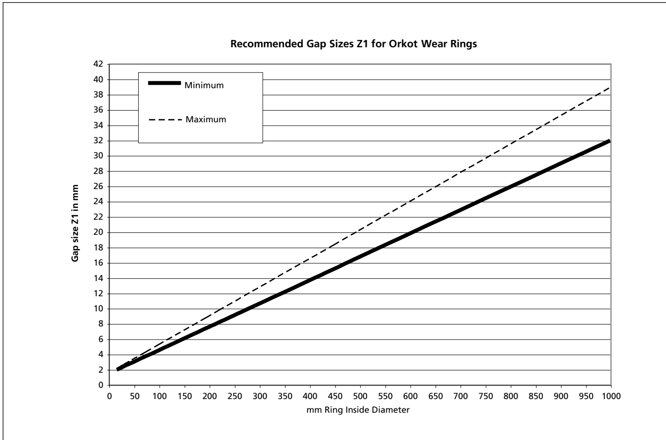
Figure 19 Recommended Gap Sizes Z1 for Orkot Wear Ring
