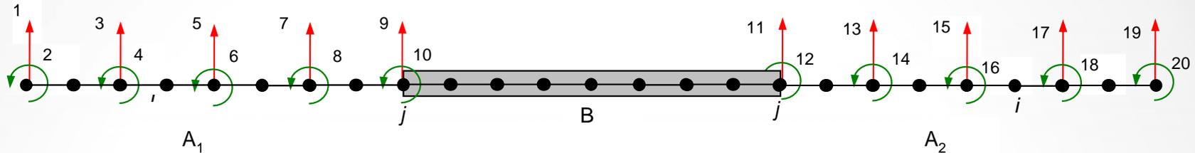
A mass of **35 grams** has been added to nodes 9 and 11 in the sub-structure B.
