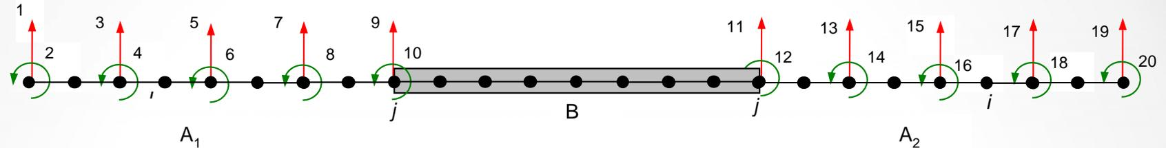
$H_{11}^C$  resulting from the coupling of  $A_1$  and  $A_2$  with the sub-structure  $B$ .
