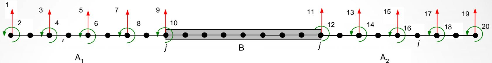
$H_{11}^C$  resulting from the coupling of  $A_1$  and  $A_2$  with the sub-structure  $B$ , with the addition of masses in  $A$
