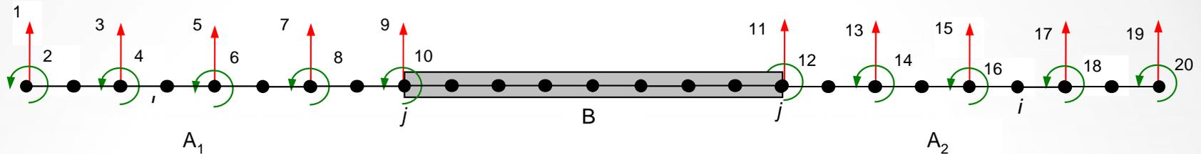
A mass of 70 grams has been added to nodes 9 and 11 in the sub-structure B.
