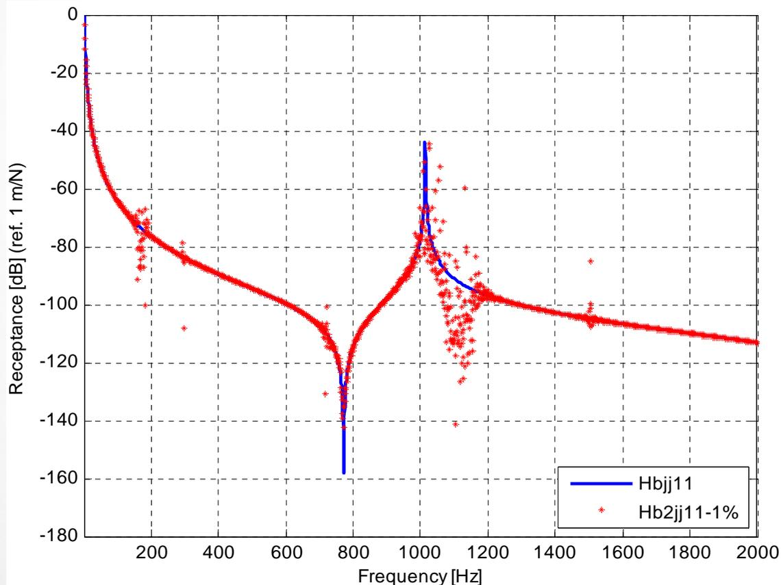
As sub-structure *B* is altered, its natural frequency changes to the left.
